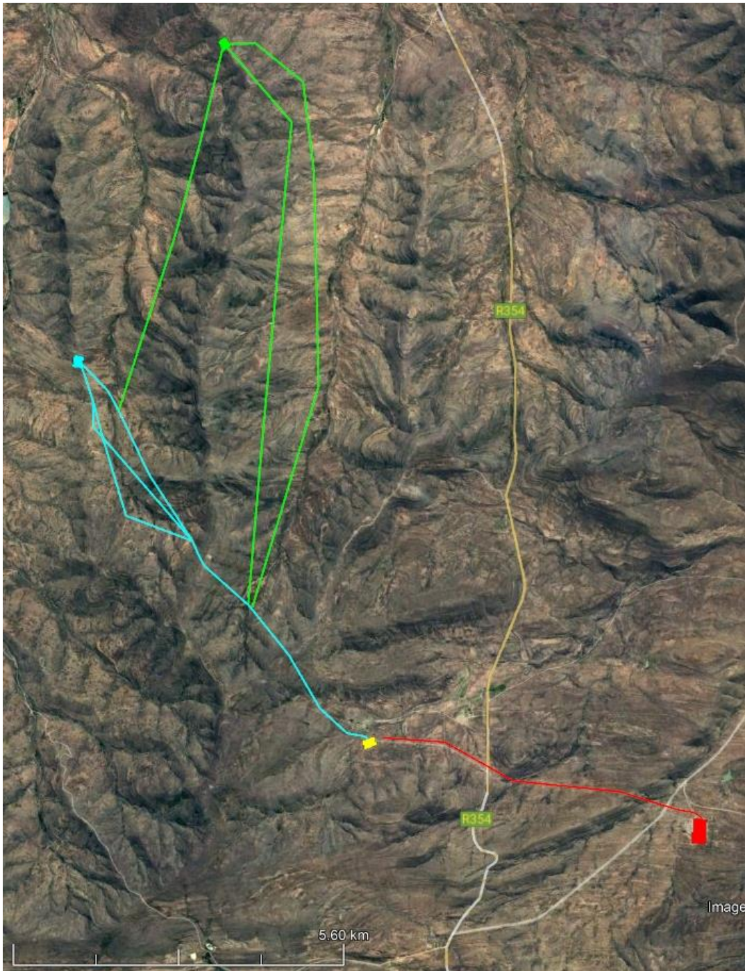
Figure 1: The proposed 132kV OHL route and substation alternatives. Green = Northern substation alternative (Option 2) with proposed grid OHL route alternatives. Blue = Southern substation alternative (Option 1) with proposed grid OHL route alternatives. Yellow = existing Bon Espirange substation. Red = existing Komsberg substation with proposed OHL route.
