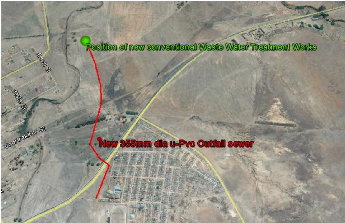
Image 2.1.2: New 355mm diameter outfall sewer line.
