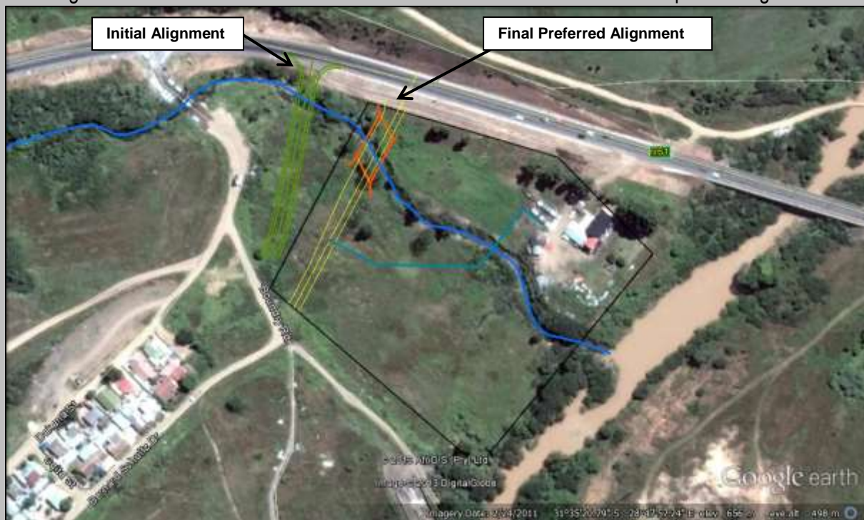
Figure 3: Alignment Alternatives Considered
