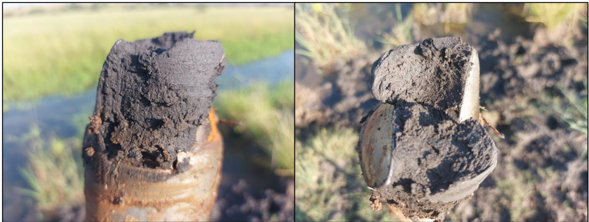
Figure 6-7 Katspruit soil form identified within the HGM 2- Floodplain wetland. The soil form consists of an orthic topsoil over a gley subsoil.
