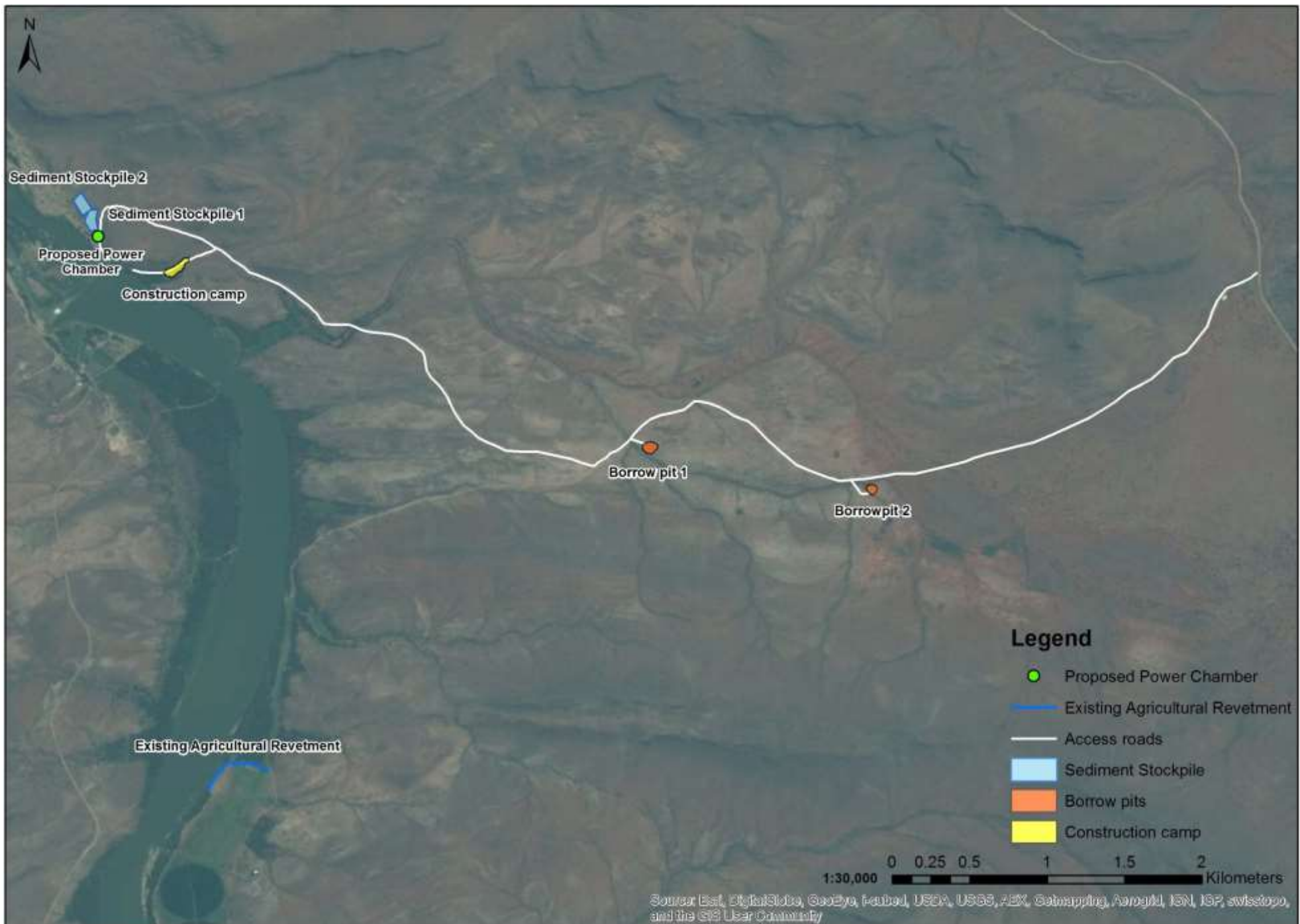
Figure 24 | Access Roads, borrow pits, construction camp, revetments and sediment storage basins for the proposed project
