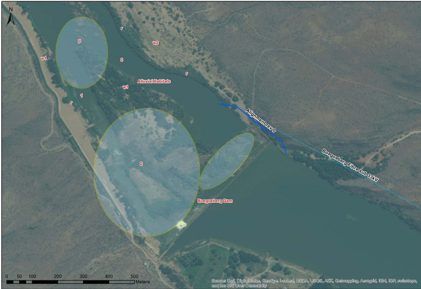
Figure 35 | Aerial view of the site to be impacted by the proposed development, showing three channels that comprise the main Orange River downstream of the dam wall, and the proposed alignment of the hydro scheme (dark blue line). Channel 1 most likely results from the permanently open sluices.
