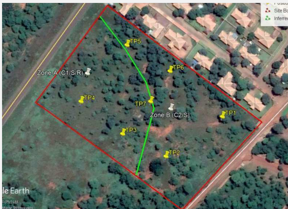
Figure 9: Geotechnical Map showing the two geological zones onsite and location of test pits
