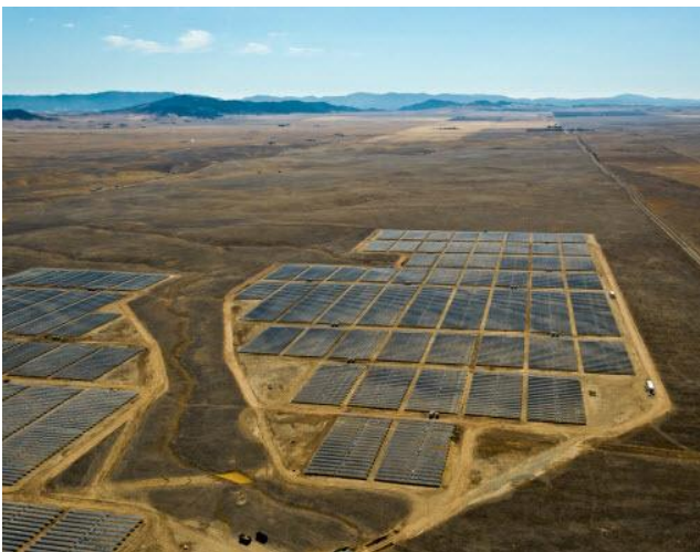
Figure 2 | Example of a PV facility in a landscape similar to Copberton needs to be converted to an Alternating Current (AC) to connect to the grid. The conventional PV and CPV technologies require significantly less water per day (19ℓ/MWh) than the CSP system which needs approximately 3,420ℓ/MWh of water per day during the operational period.
