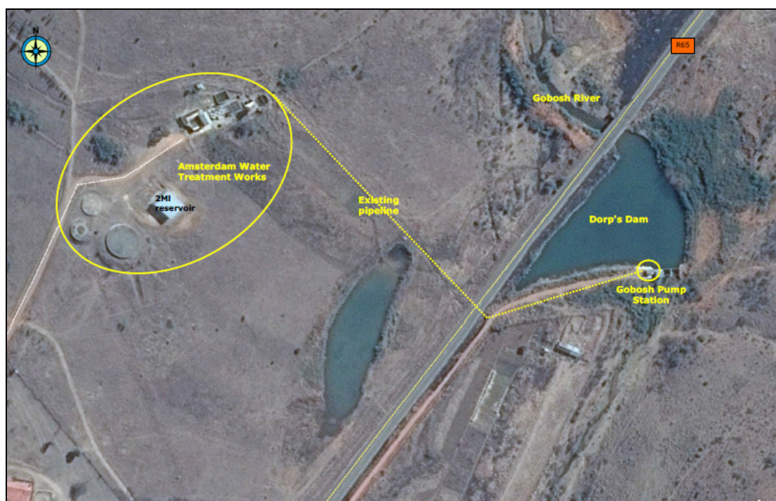
Figure 5.1: Amsterdam Water Treatment Works and associated infrastructure
