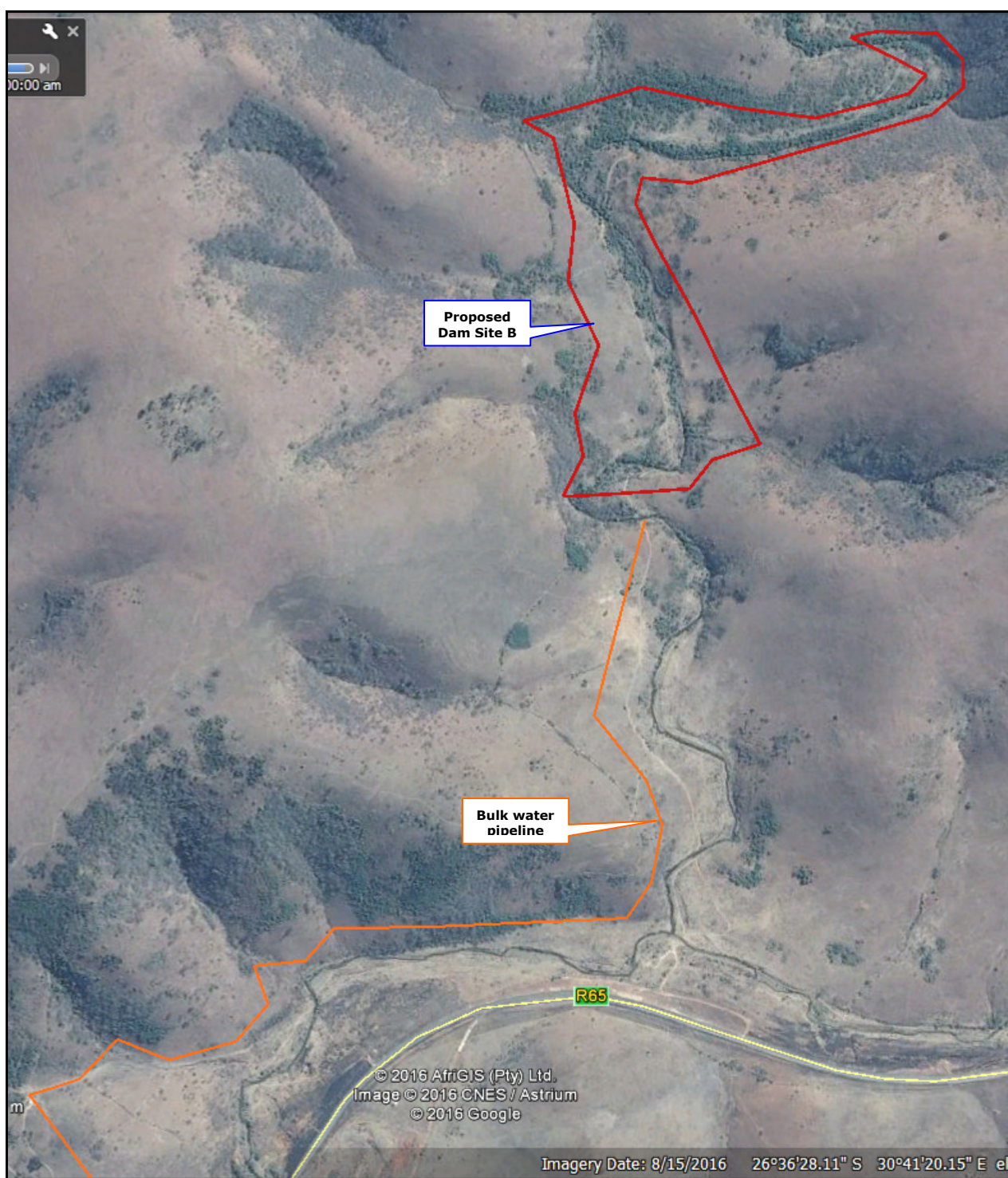
Figure 3.7b: Aerial view of Dam Site B and bulk water pipeline.
