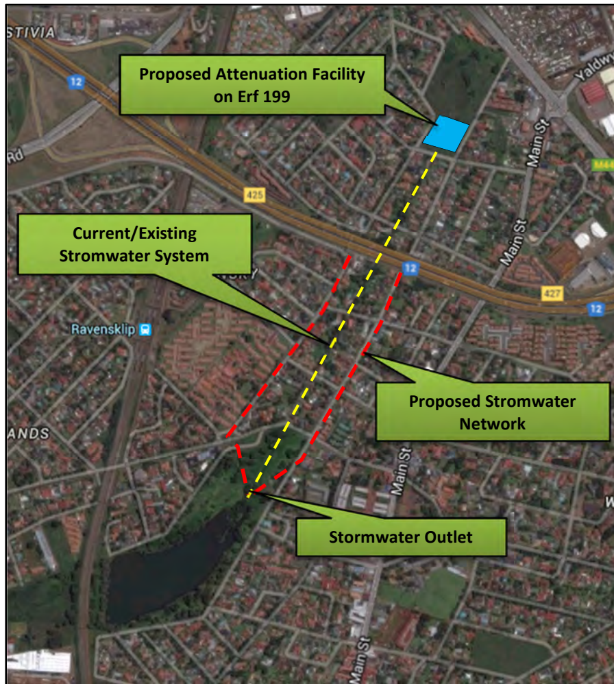
Figure 0- 1 Proposed Stormwater Network and Attenuation Pond
