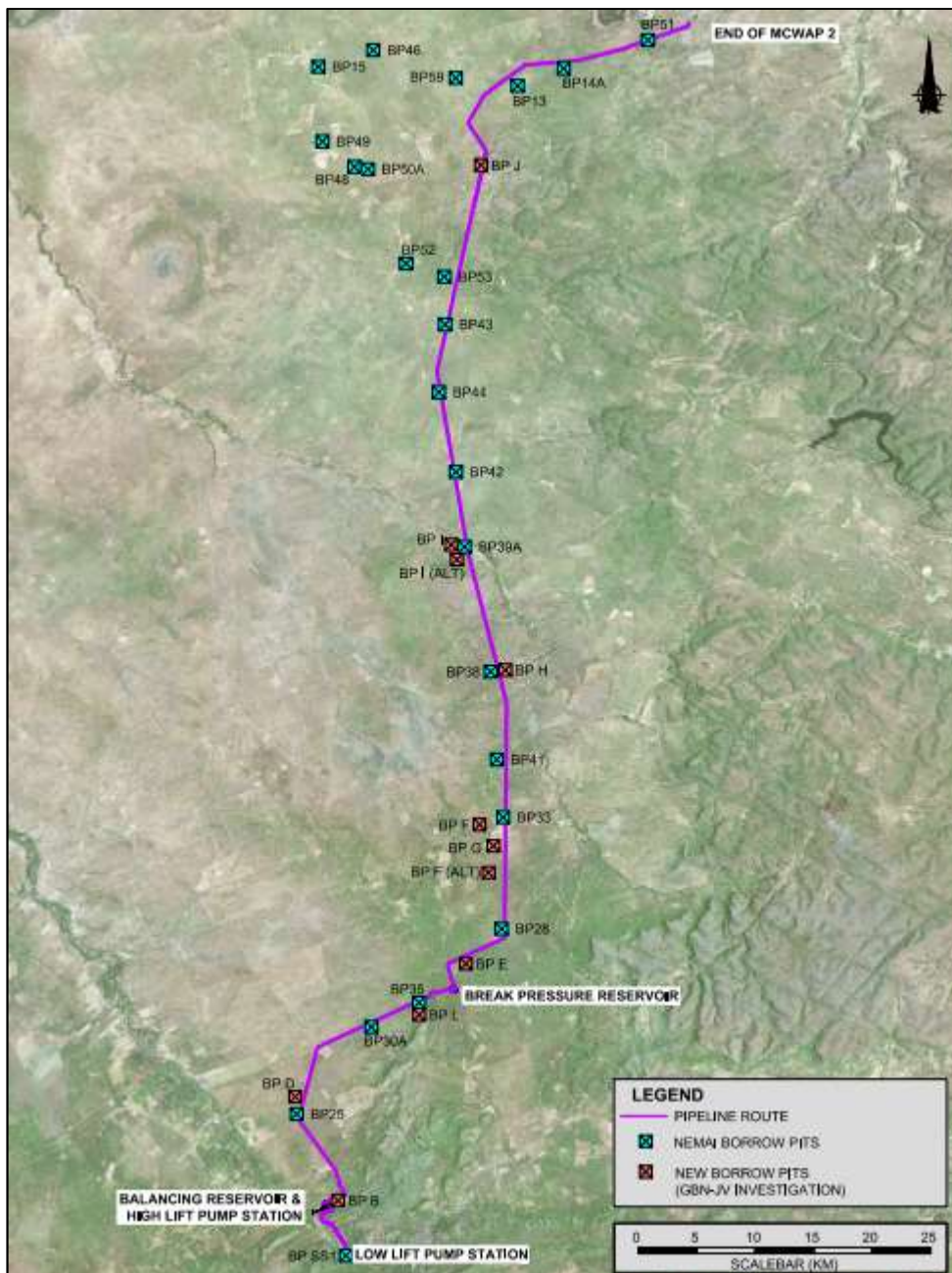
Figure 3: MCWAP-2 Project including the pipeline (purple), the NEMA borrow pits (blue) and the additional GBN-JV borrow pits (red)
