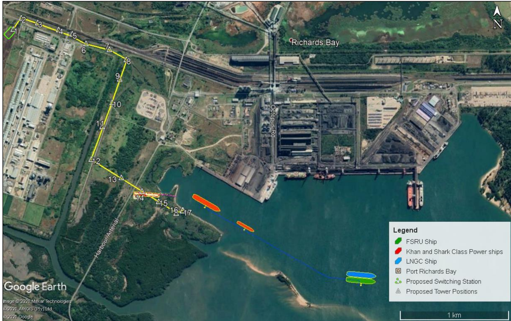
Figure 1-1: Google image showing the Gas to Power via Powership Project (preferred alternatives) – Port of Richards Bay
