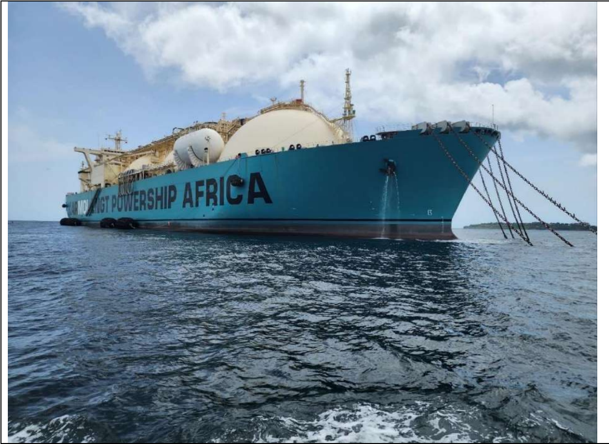
FSRU secured with vessel spread mooring system
