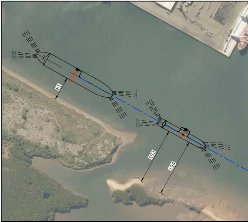
Figure 1-6: Powerships' distance from the sandspit /shore (in meters) Figure 1-7: FSRU distance from the sandspit (in meters)
