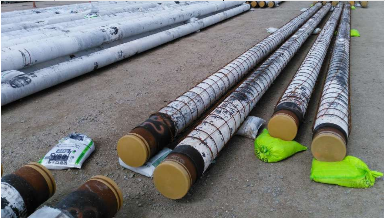
Steel pipes with concrete weight coating in various stages of fabrication pre-installation on the sea bed
