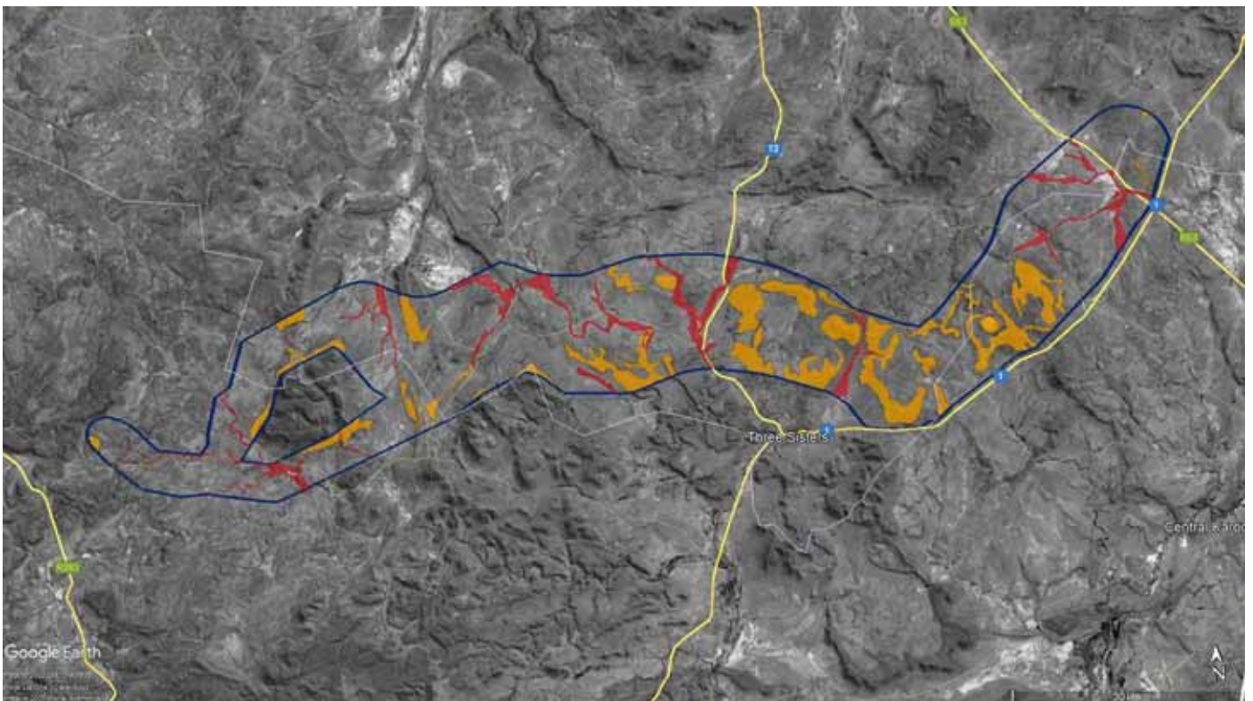
Figure 30: Ecological constraints map for physical infrastructure and roads in the Gamma Grid Assessment Corridor (red = No-Go areas, orange = High Sensitivity areas).
