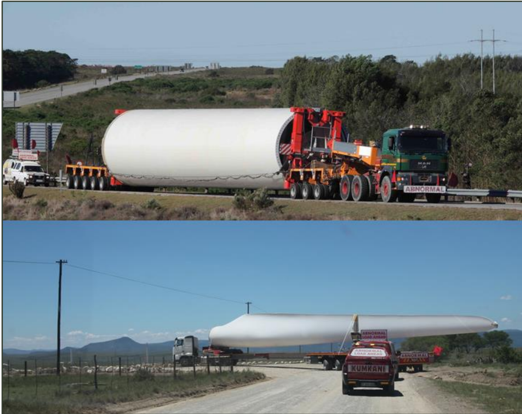
Figure 6.8: Tower section in low load configuration shown in top photo; and blade shown in bottom photo
