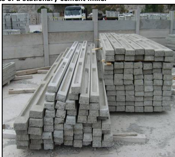
Photo 3.5: An example of a lintel mould/casting bed and the final product
