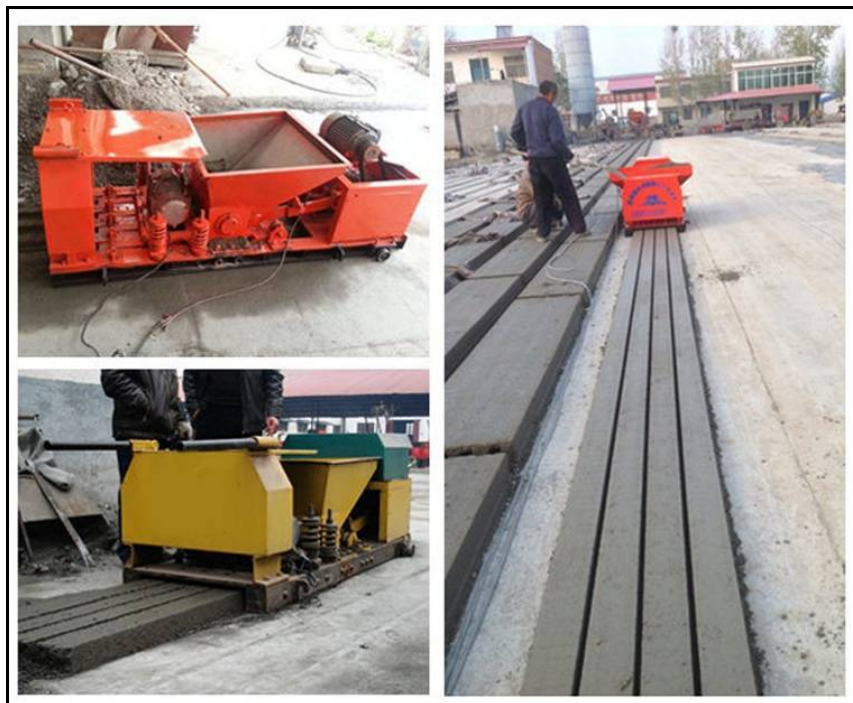
Photo 4.1: Automated lintel manufacturing process
