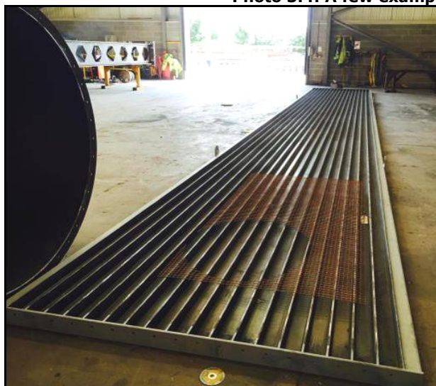
Photo 3.5: An example of a lintel mould/casting bed and the final product
