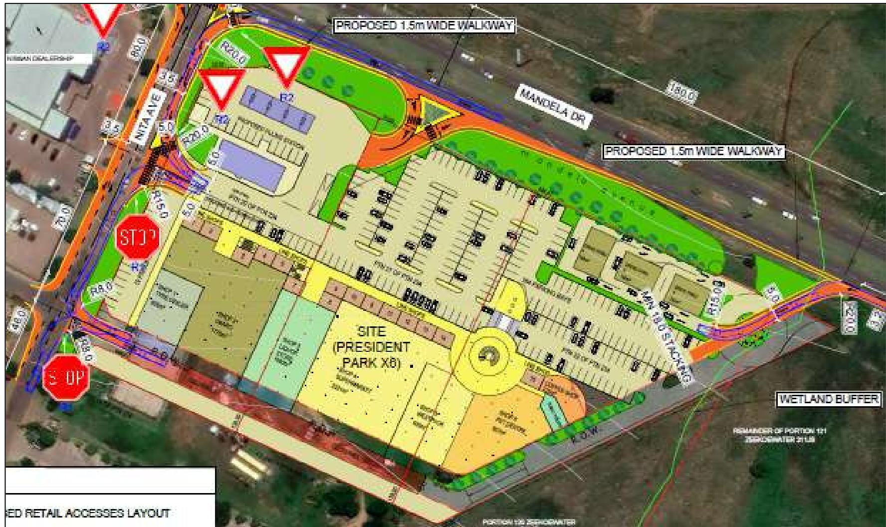
Figure 7.6: Alternative layout 3 (re-aligned access road from Mandela Drive) (designed by Michael M. Payne & Associates Architects, 2020)
