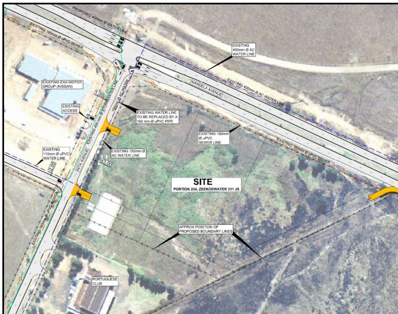
Figure 7.8: Location of the existing municipal water and sewer infrastructure adjacent to the site (taken from WSP SA Civil and Structural Engineers (Pty) Ltd., 2010)
