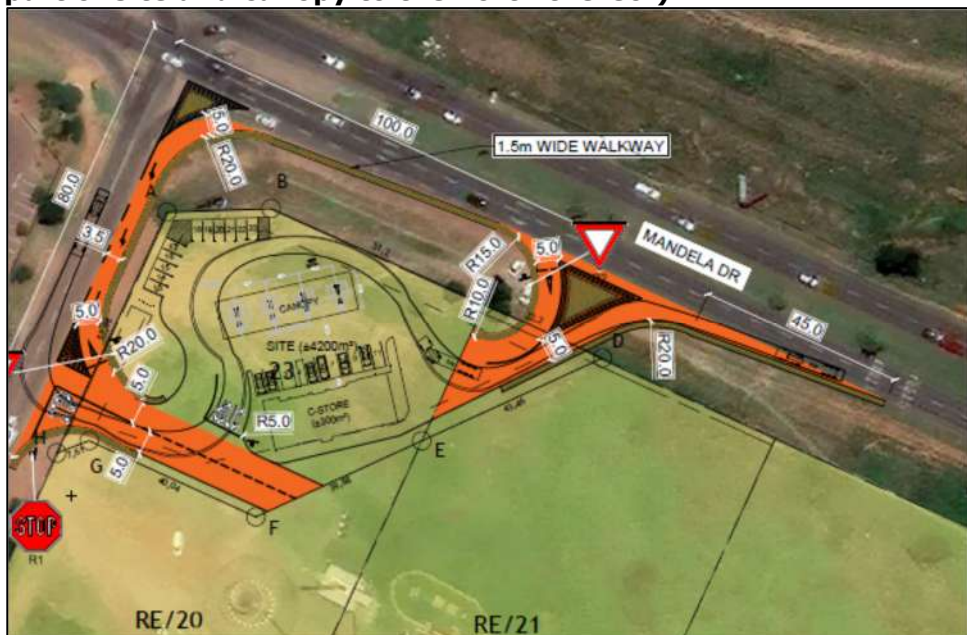
Figure 7.4: Alternative layout 2 (convenience store and canopy moved to provide for turning of fuel tankers)
