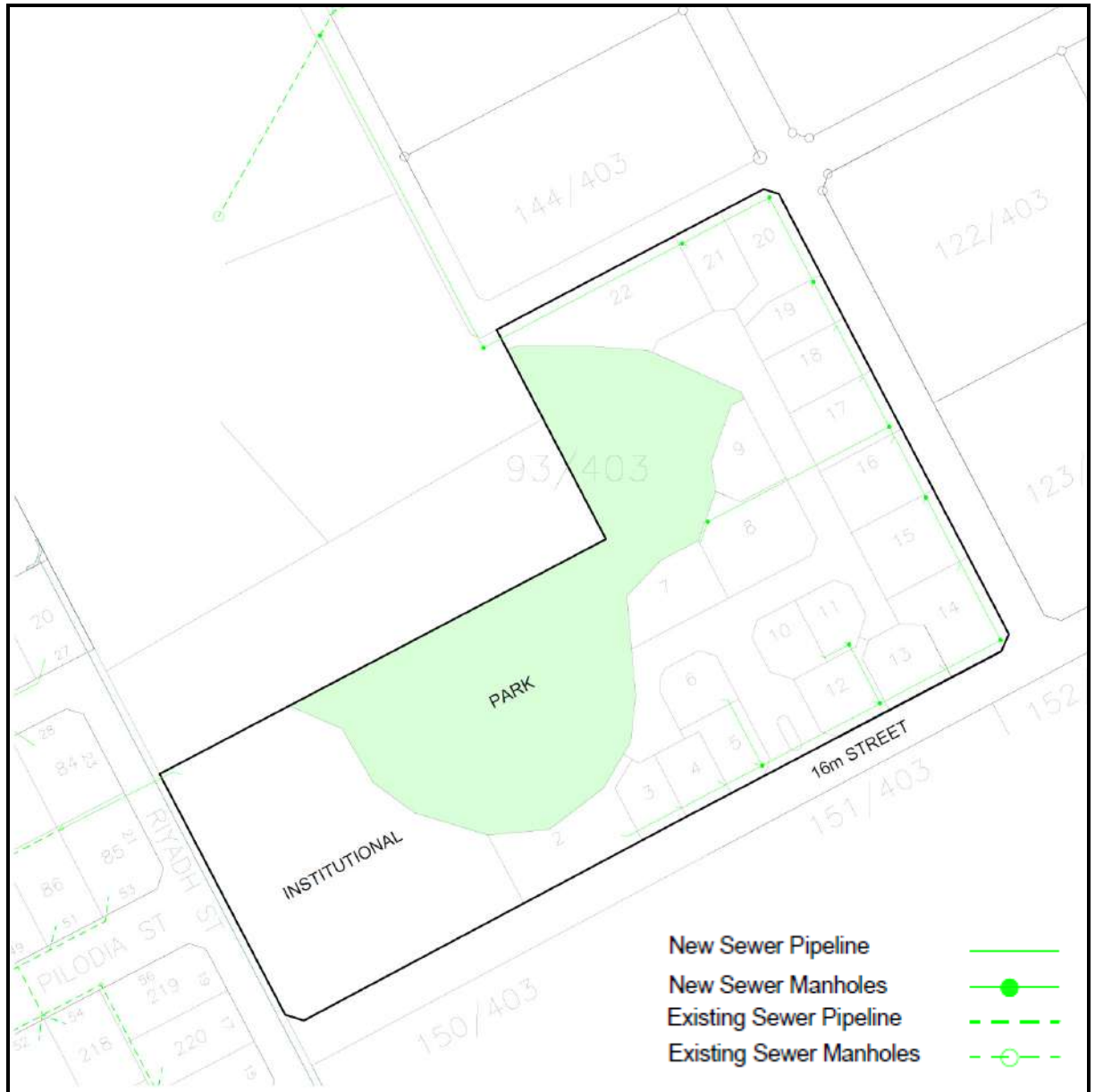
Figure 3.4: Sewer reticulation network (taken from Bower, 2018a)
