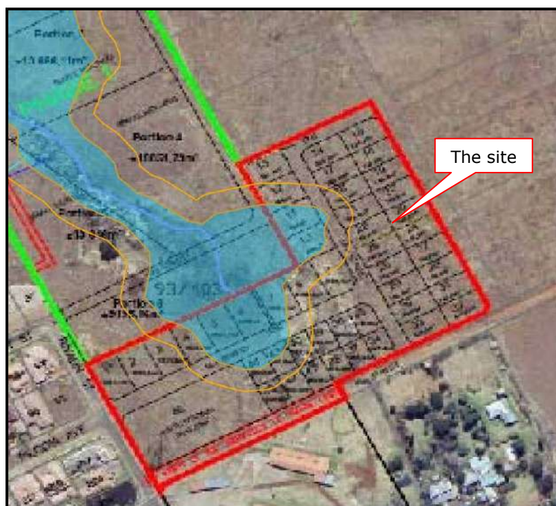
Figure 7.2: Layout plan 1 indicating wetland and 20m wetland buffer zone (taken from Davis, 2012)
