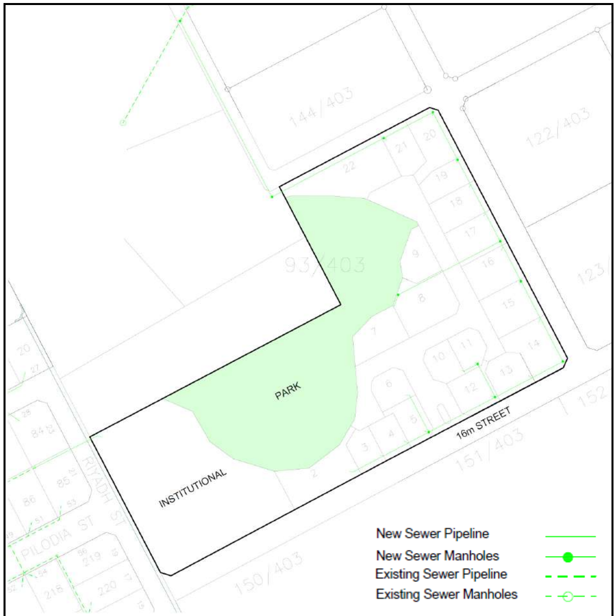
Figure 3.4: Sewer reticulation network (taken from Bower, 2018a)
