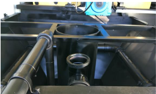
Containerised and tank unit clarifier (humus tank).
