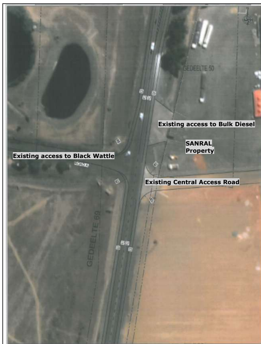
Figure 7.1: Alternative layout 1 (use existing access road directly from R35) (taken from Roberts, 2019).
