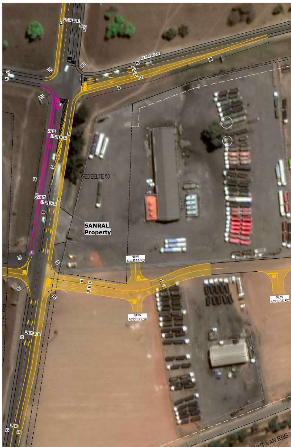
Figure 7.2: Alternative layout 2 (realign existing access road directly from R35) (taken from Roberts, 2019).
