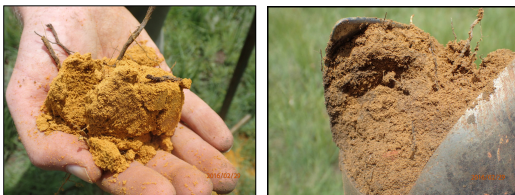
Figure 5.10b: Illustrates examples of distinct yellow colours in the yellow-brown apedal B-horizon (left) and multi-colourness in the orthic A-horizon (right), recorded within the study area (taken from Grobler, 2016).
