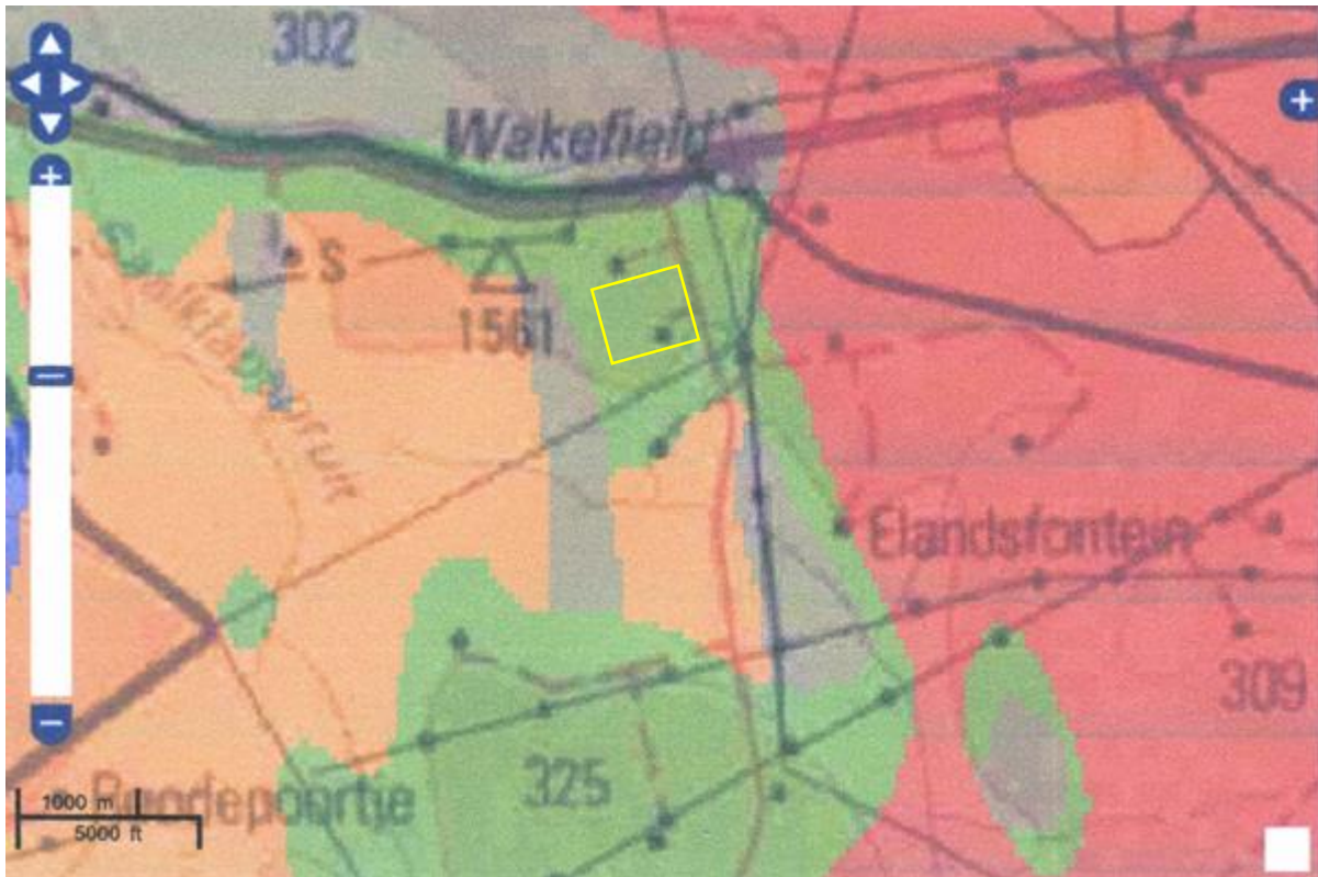
Figure 8-55 : SAHRIS palaeosensitivity map for the site for the proposed cemetery shown within the yellow rectangle. Background colours indicate the following degrees of sensitivity: red = very highly sensitive; orange/yellow = high; green = moderate; blue = low; grey = insignificant/zero.
