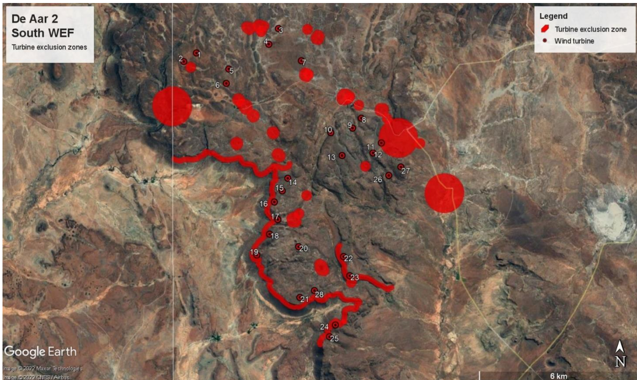
Figure (iii): The proposed turbine exclusion positions for Jackal Buzzard nests, boreholes, dams and escarpment edge. It has been confirmed by the specialist that all 28 positions are outside of these recommended exclusion zones
