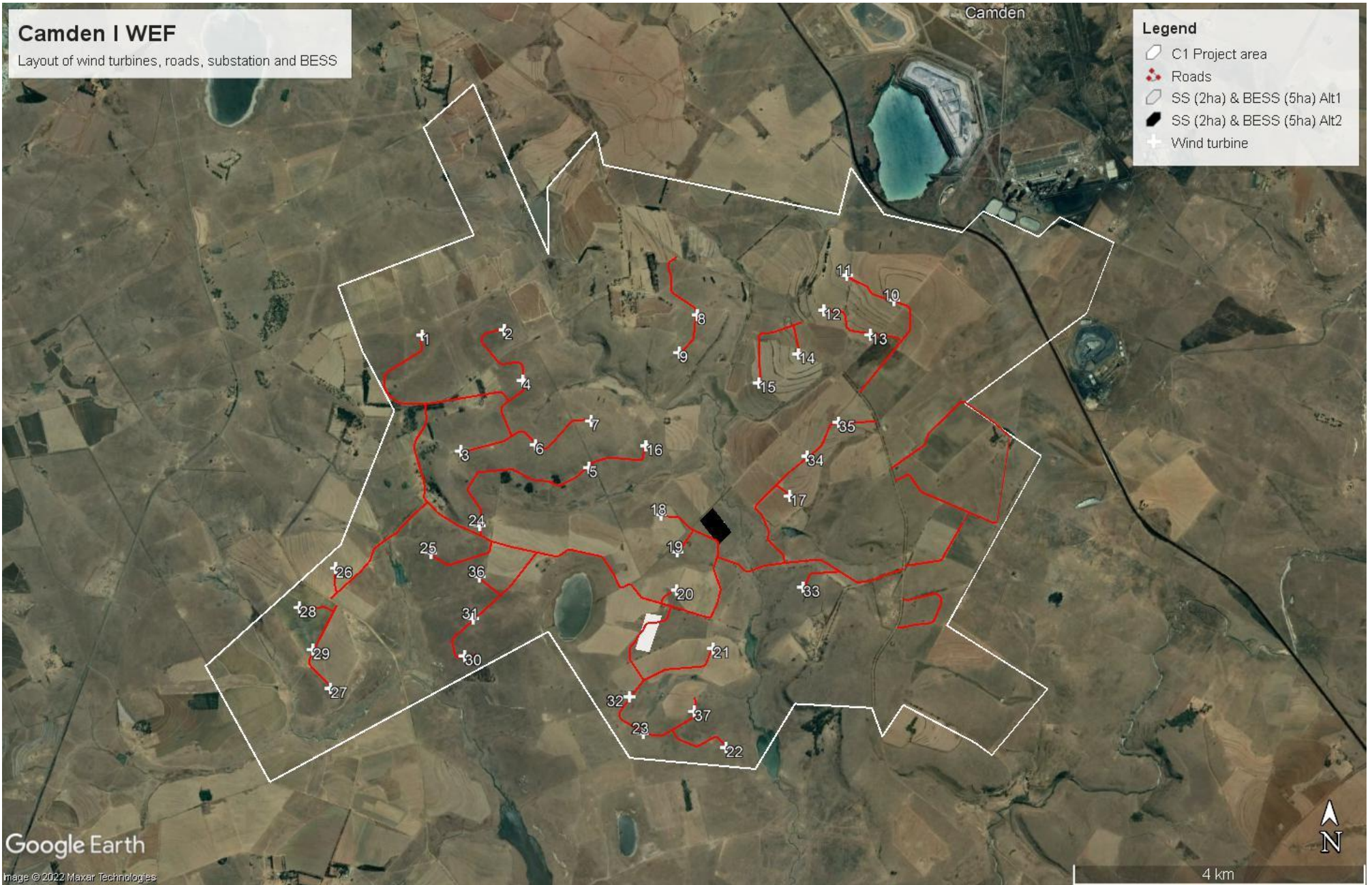
Figure 1: Proposed layout of the project area of the proposed Camden I WEF and BESS alternatives.
