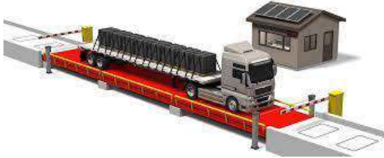
Image 11: Typical Weighbridge that will be constructed. (Synman, 1998)
