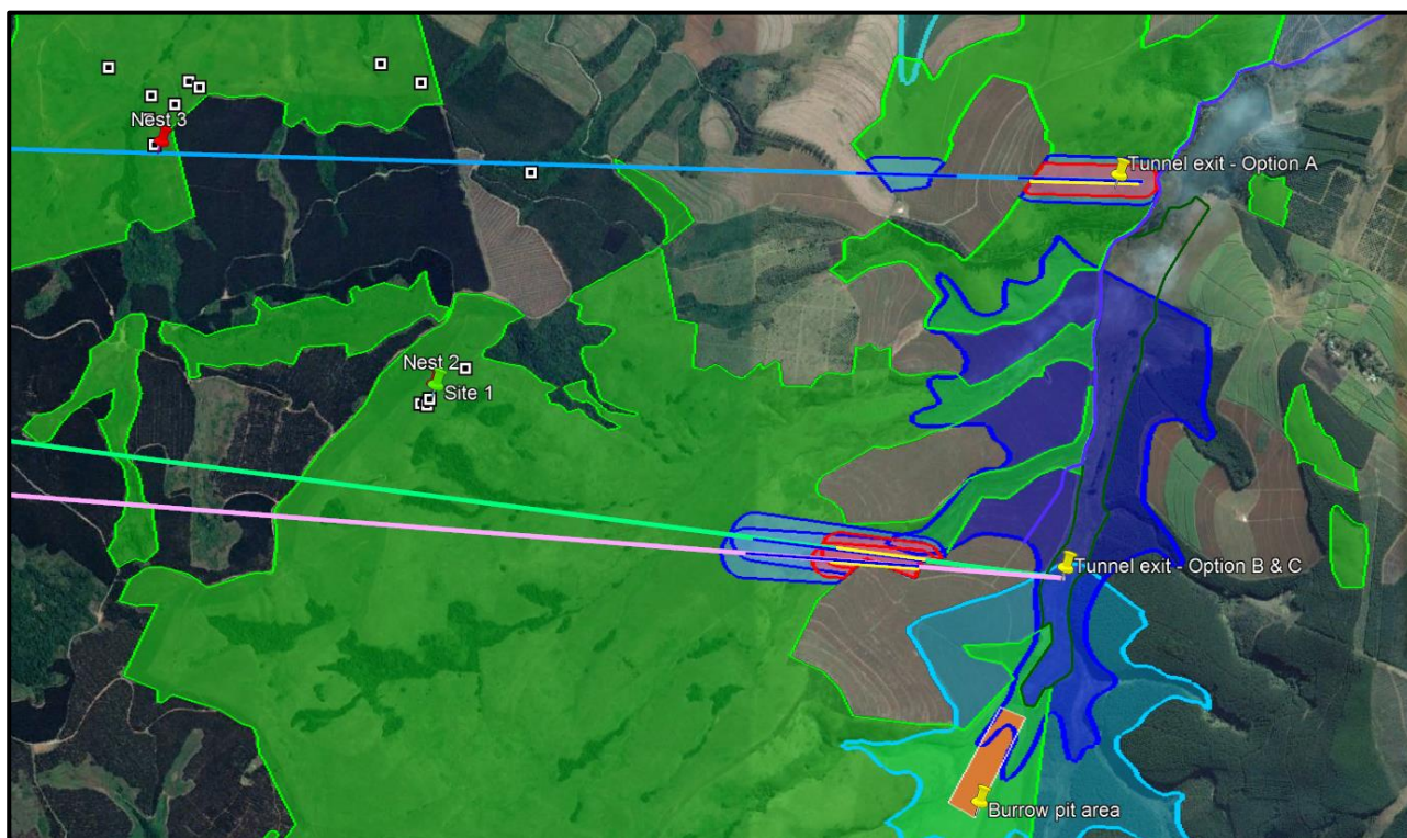
Figure 12: Positions along the tunnelling alignment which lies within the TBM vibration radius of influence (Kroch & Heyns 2018)
