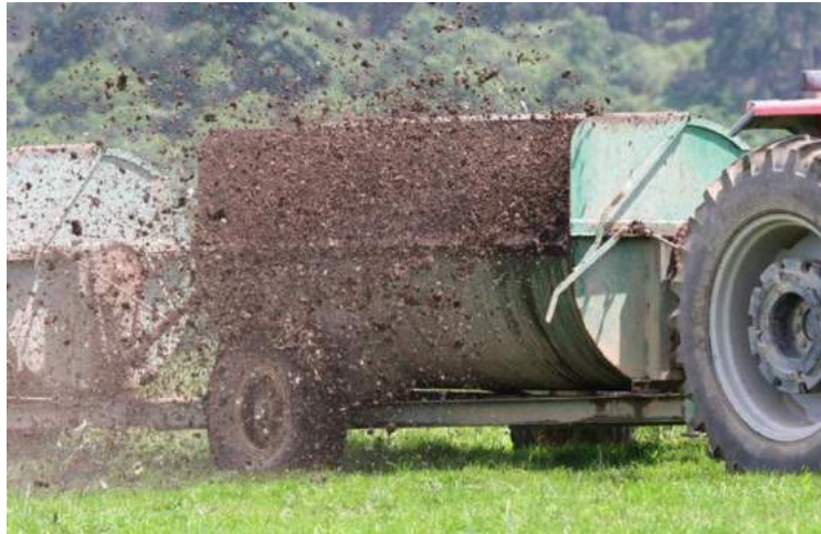
Figure 20: Typical Rotor-spreader “Muck” spreader used on the Brookdale Farm
