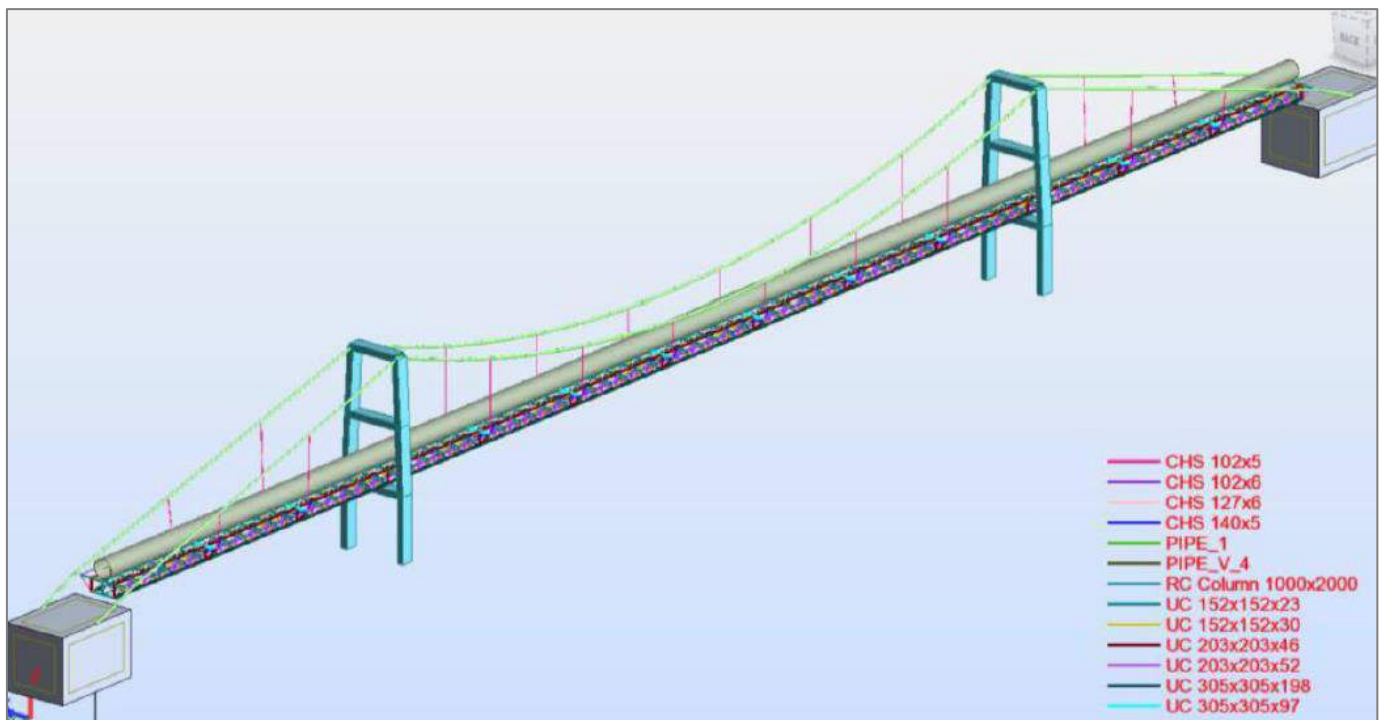
Figure 62: Three-Dimensional View of Suspension Bridge
