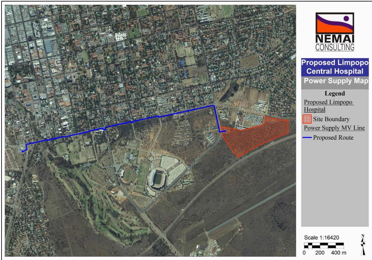
Figure 11: Proposed Power Supply 11kV Cable Route from the Beta Substation to the Proposed Site
