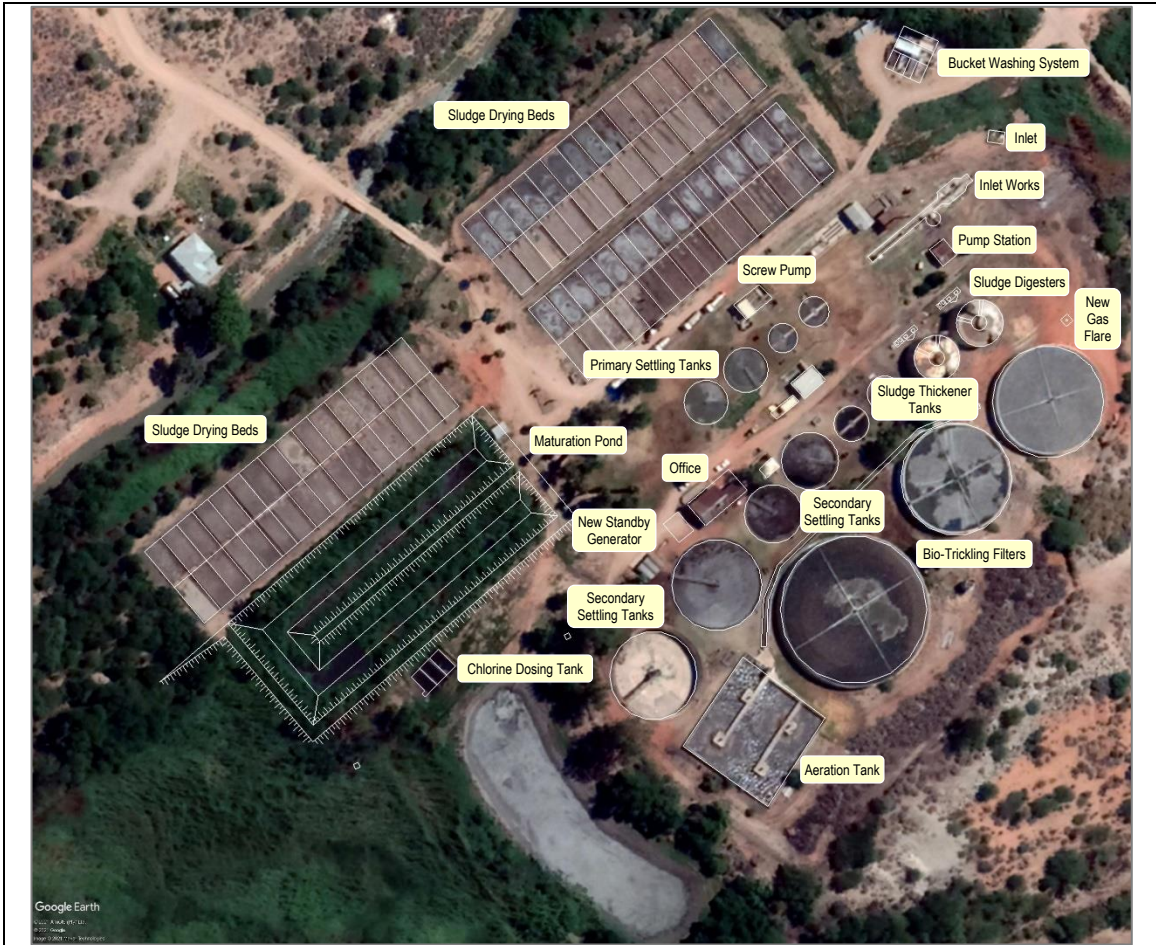
Figure 2: K-WWTW existing infrastructure to be refurbished (Google Earth image) (Note: not all infrastructure is labelled in the map above due to scale)
