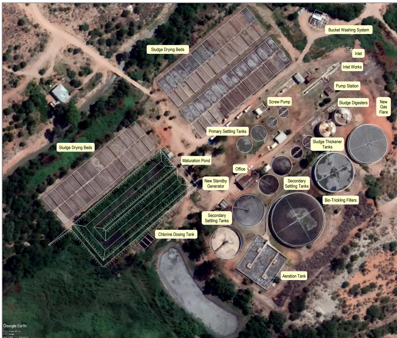
Figure 6: K-WWTW existing infrastructure to be refurbished (Google Earth image) (Not all infrastructure is labelled in the map above due to scale – see full details in map in Appendix D1 )
