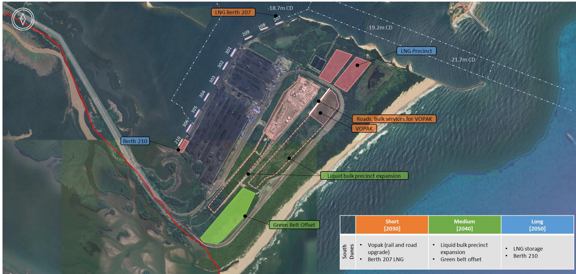
Figure 7: Revised version of PoRB Master Plan showing the proposed end state of South Dunes Precinct
