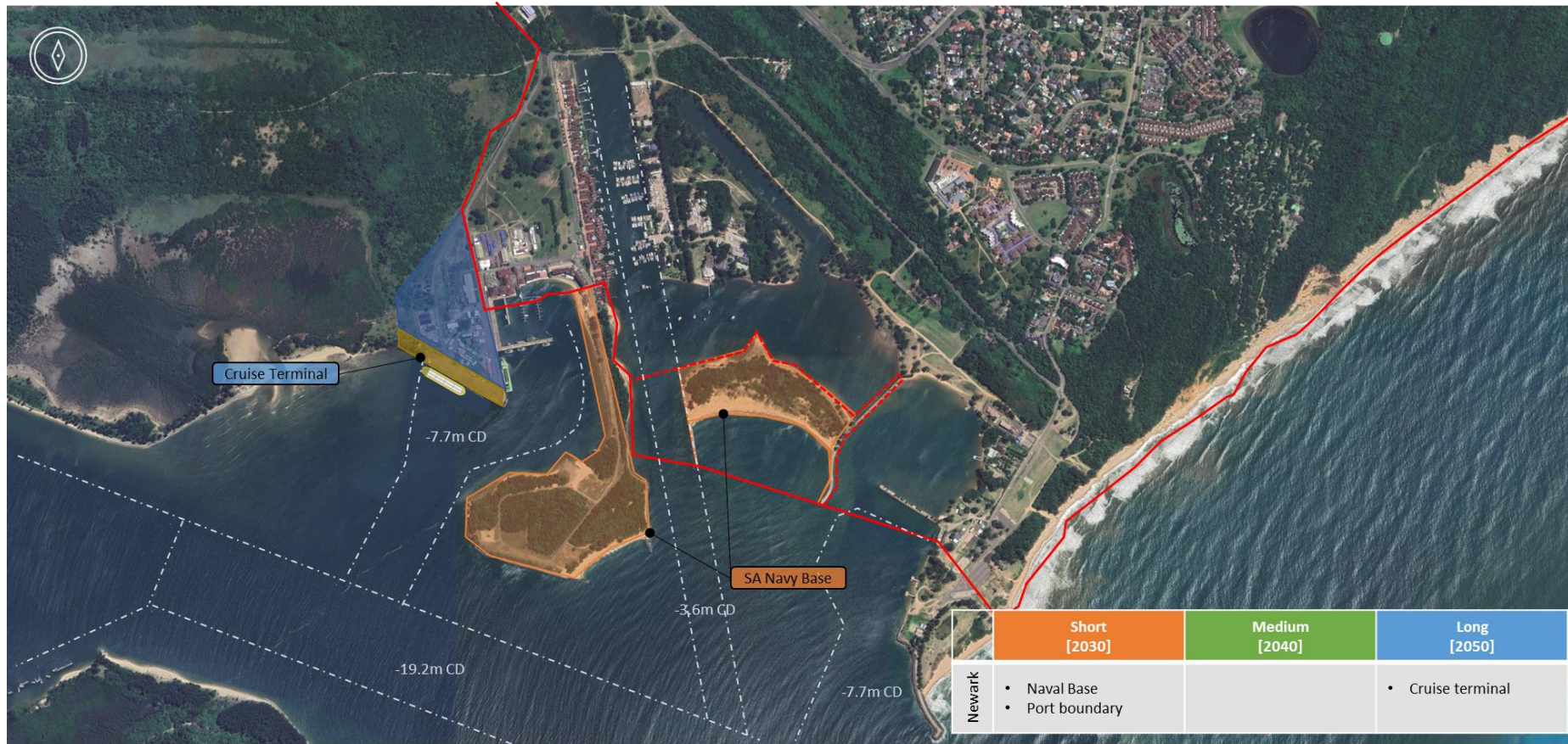
Figure 8: Revised version of PoRB Master Plan showing the proposed end state of Newark Precinct
