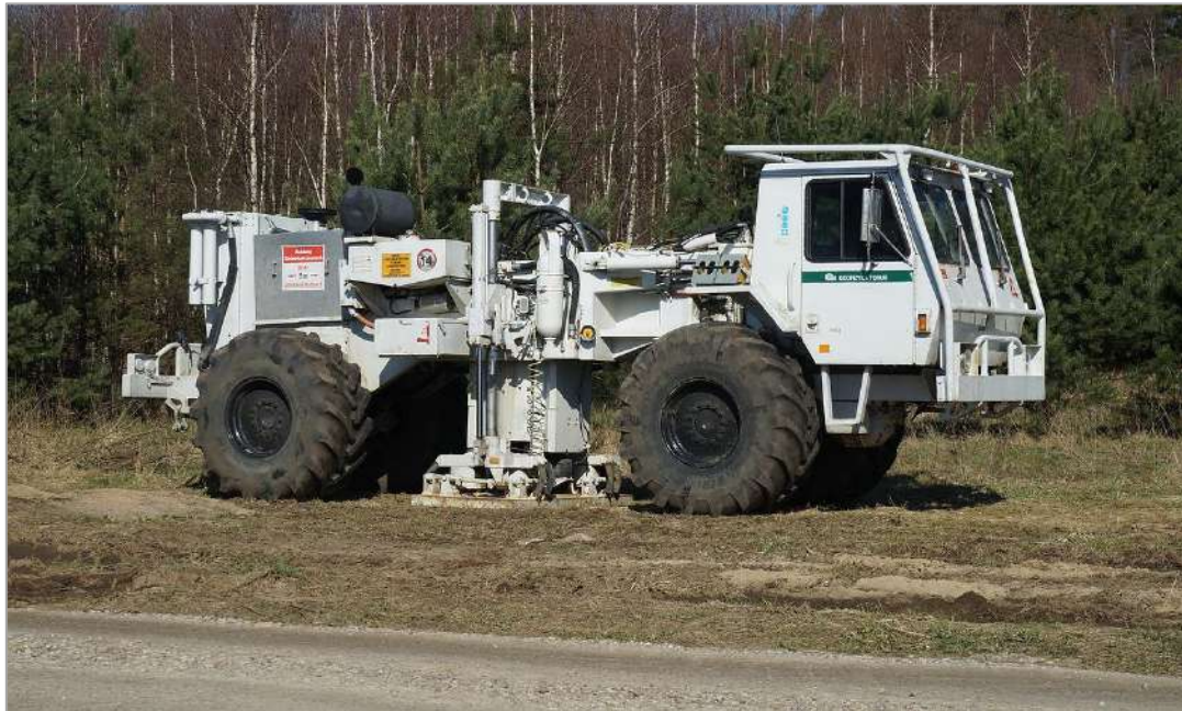
Figure 10: Example of a vibroseis truck
