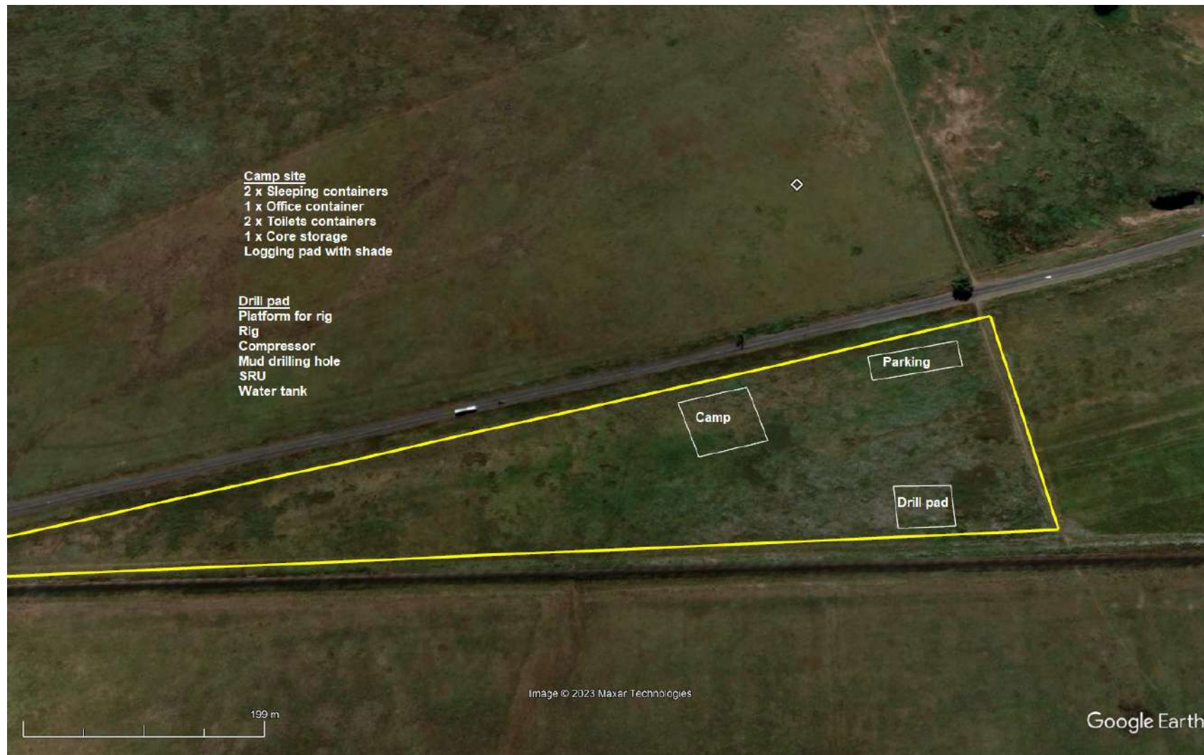
Figure 9: Schematic of proposed drill site
