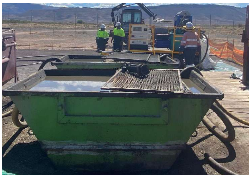
Figure 88: Example of storage tanks used to manage drilling fluids
