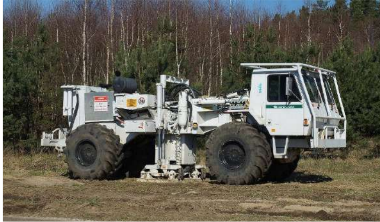
Figure 5: Example of a Vibroseis truck (Nemai, 2023)
