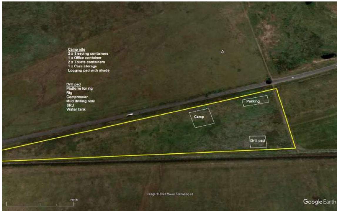
Figure 2 Borehole Drilling Site Layout
