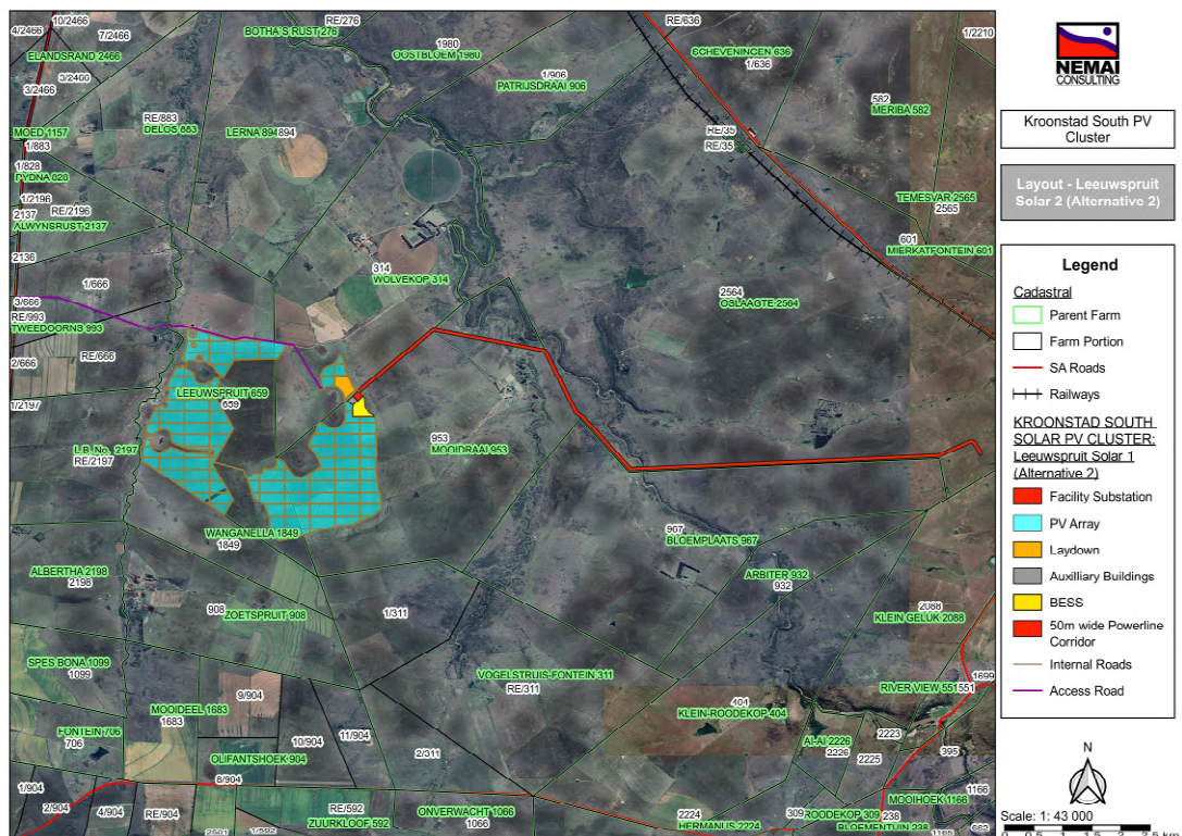
Figure 2: Locality map for Layout Alternative 2 (including PV Site, Power Line and Substation)
