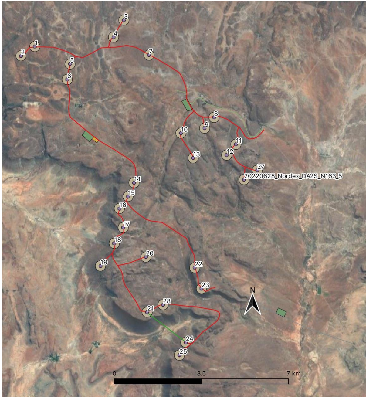
Figure 2: Final layout plan of the Mulilo De Aar 2 South WEF east of De Aar, showing WTG positions and hardstand buffers (numbered dots), internal roads (red lines), 33 kV internal reticulation (green line), construction laydown areas (green polygons) and on-site substation (yellow polygon).
