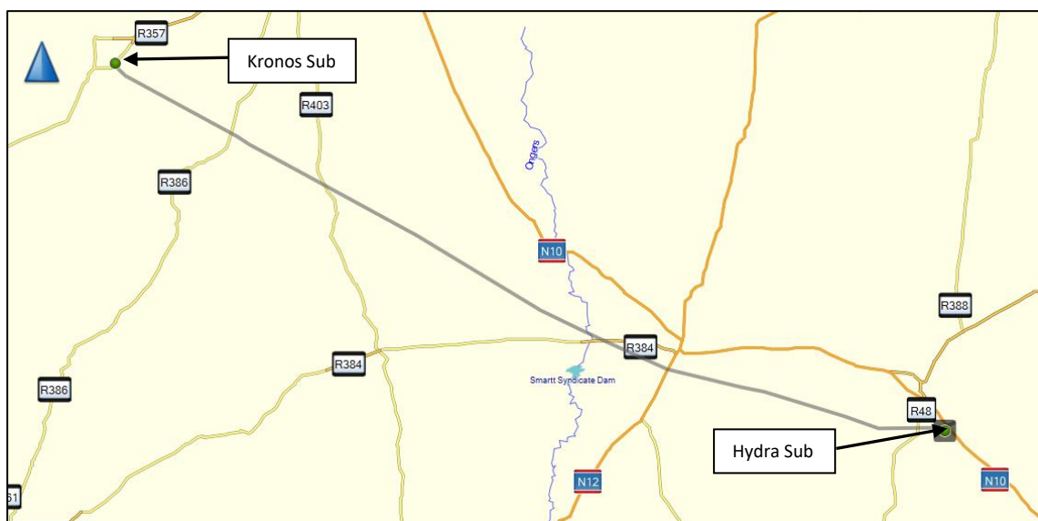
Figure 1.1: Map of the study area (Hydra Substation to the Kronos Substation) between De Aar and Copperton (Northern Cape Province). The proposed corridor of the power line is represented by the grey line.
