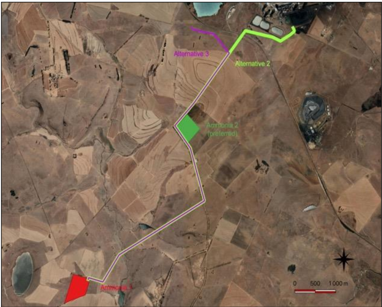
Figure 11: Pipeline alternatives for Ammonia 1.
