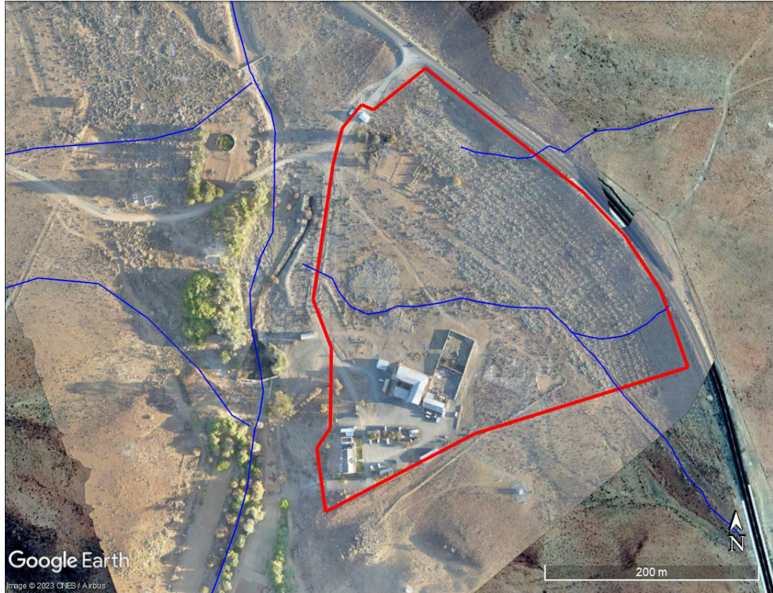
Figure 8-1: Location and extent of the watercourses within the project site
