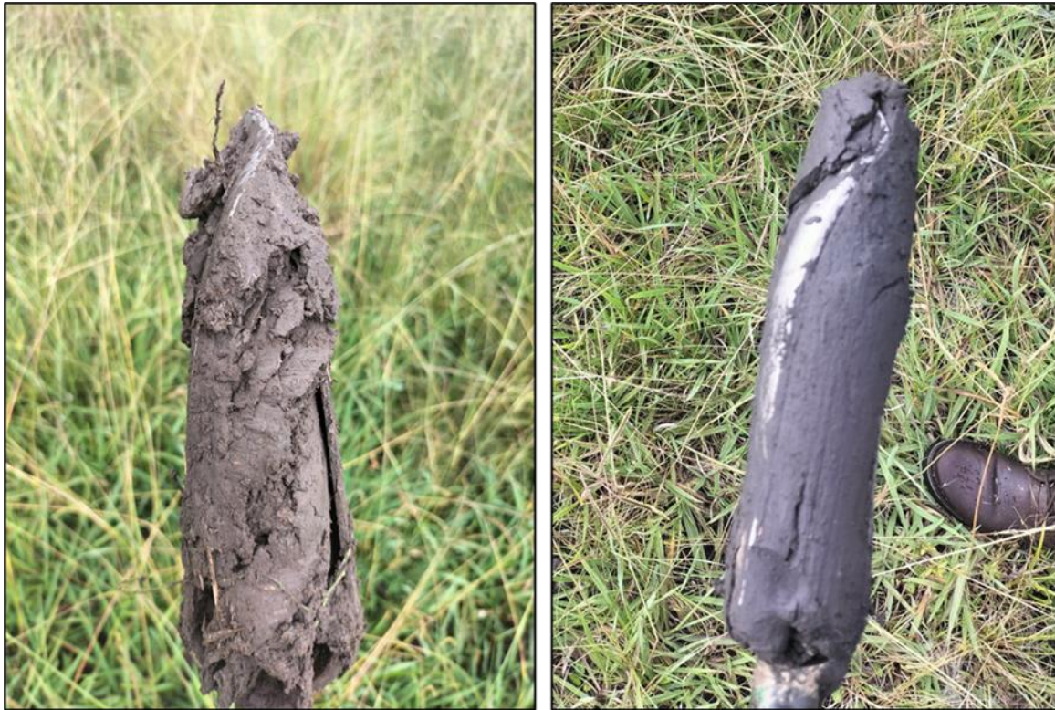
Figure 14: Photographic representation of the soils within the EA landtype displaying strongly structured, high clay content, dark brown soils.
