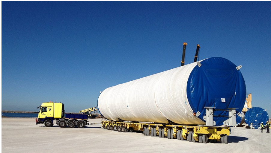
Figure 4-3:Transporting the Tower Sections (Montiea, 2014)
