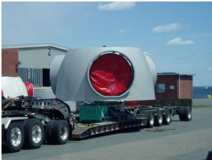
Figure 4-4:Transporting the rotor hub (Richardstransport, n.d.)
