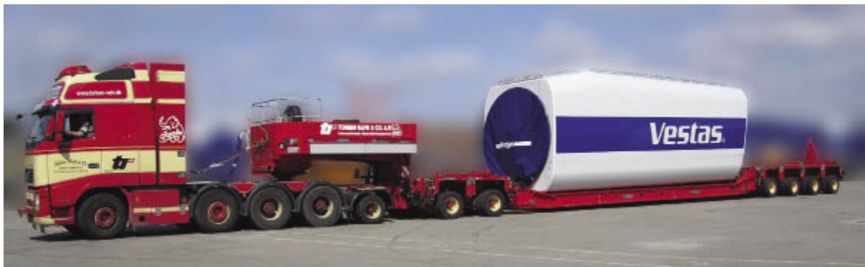
Figure 4-1:Transporting the Nacelle (Dvorak, 2010)
