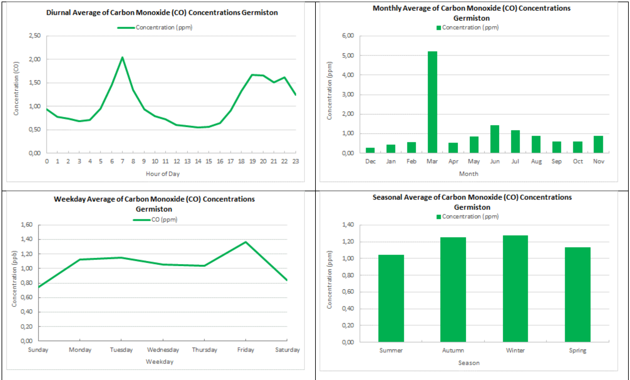
Figure 4-8: Average Diurnal, Weekday, Monthly and Seasonal CO Concentrations (ppm) for the Period January 2011 to December 2016.
