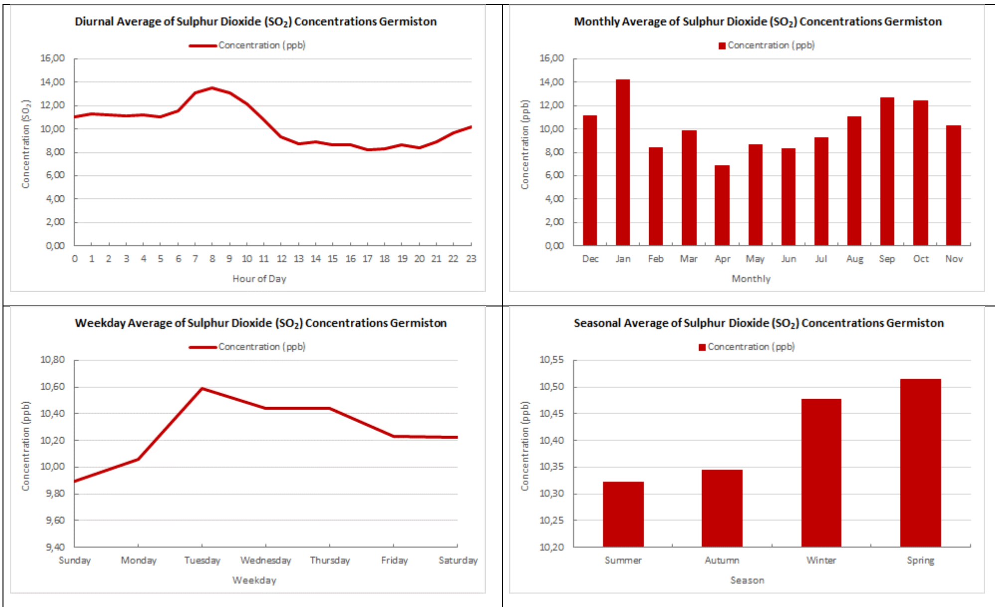
Figure 4-14: Average Diurnal, Weekday, Monthly and Seasonal SO 2 Concentrations (ppb) for the period January 2011 to December 2016.
