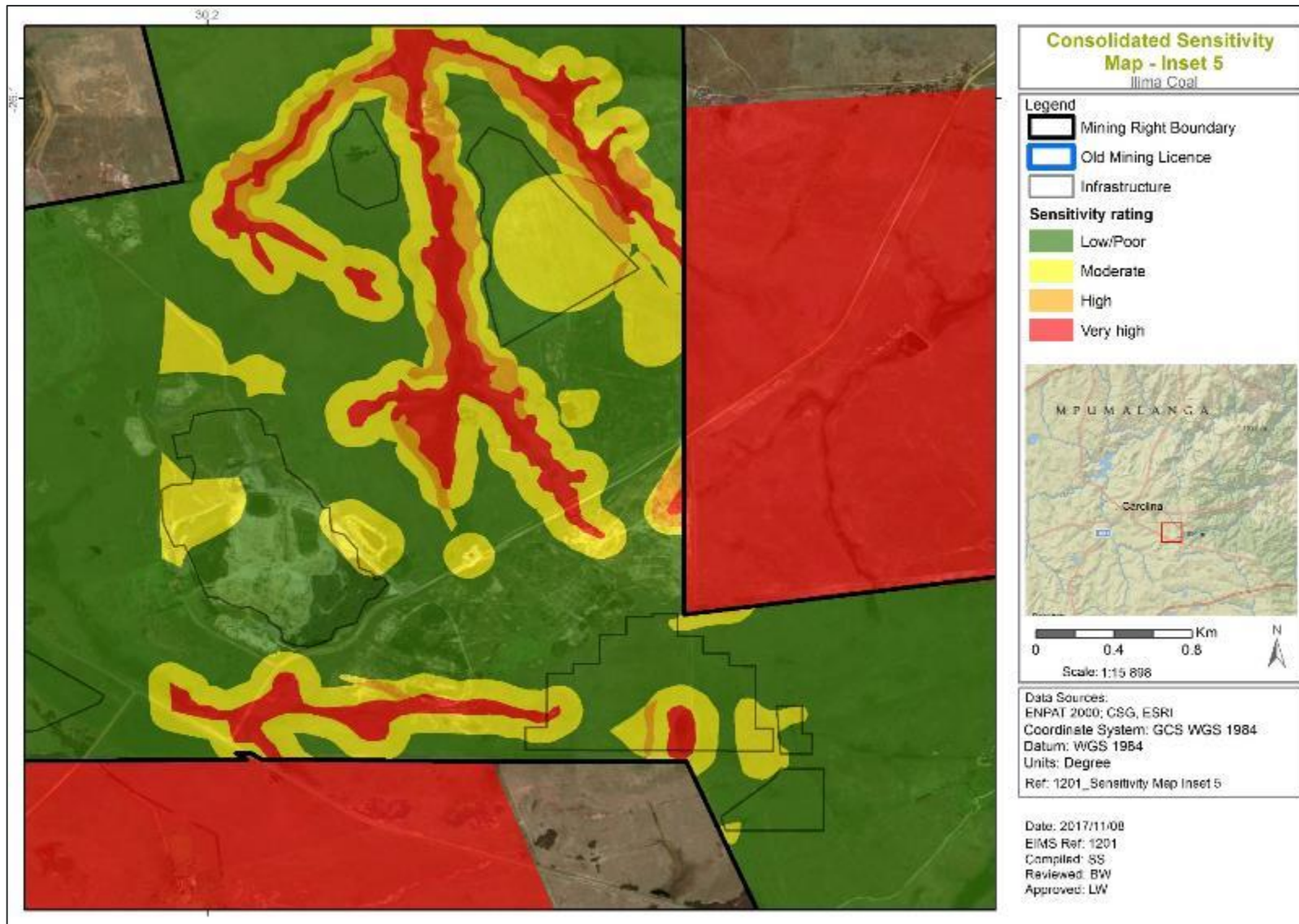
Figure 44: Sensitive environmental features and mine infrastructure map (Inset 5).
