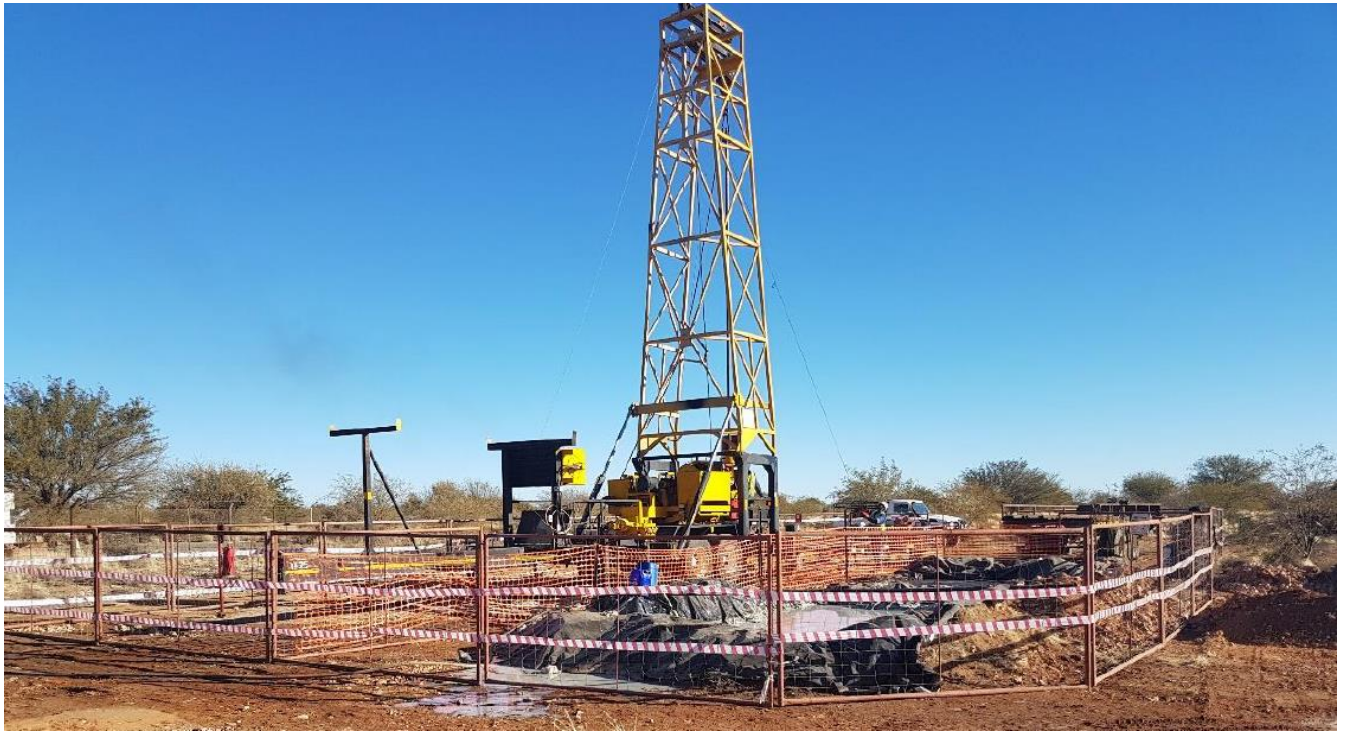
FIGURE 3-1: TYPICAL DIAMOND-CORE DRILLING RIG
