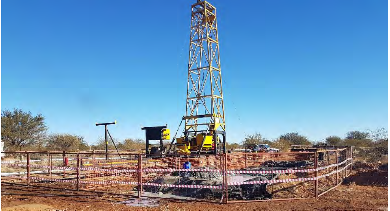
FIGURE 3-1: TYPICAL DIAMOND-CORE DRILLING RIG
