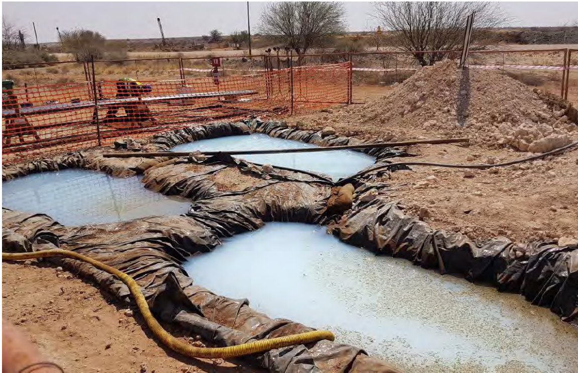
FIGURE 29-1: SETTLING PONDS USED FOR THE RECYCLING OF WATER AT A DRILLING RIG
