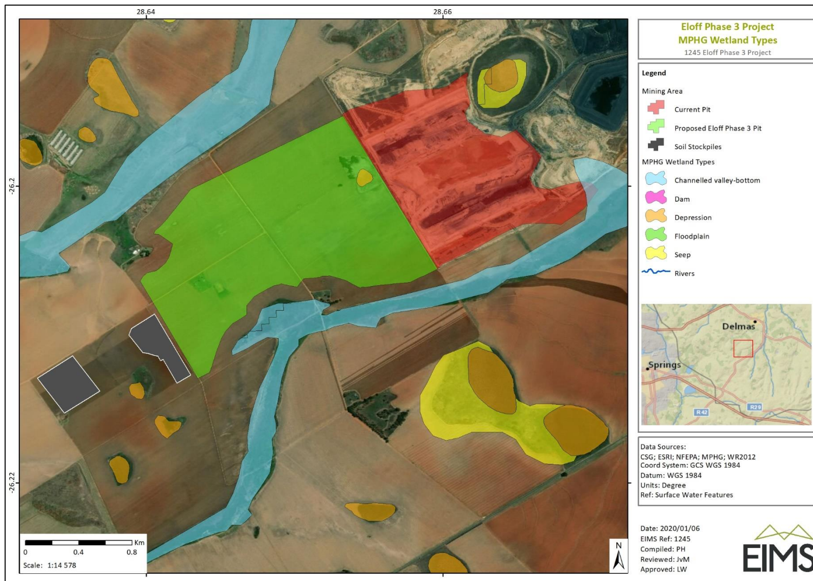
Figure 25: The FEPA and MGHG wetland types within and around the Phase 3 Project area
