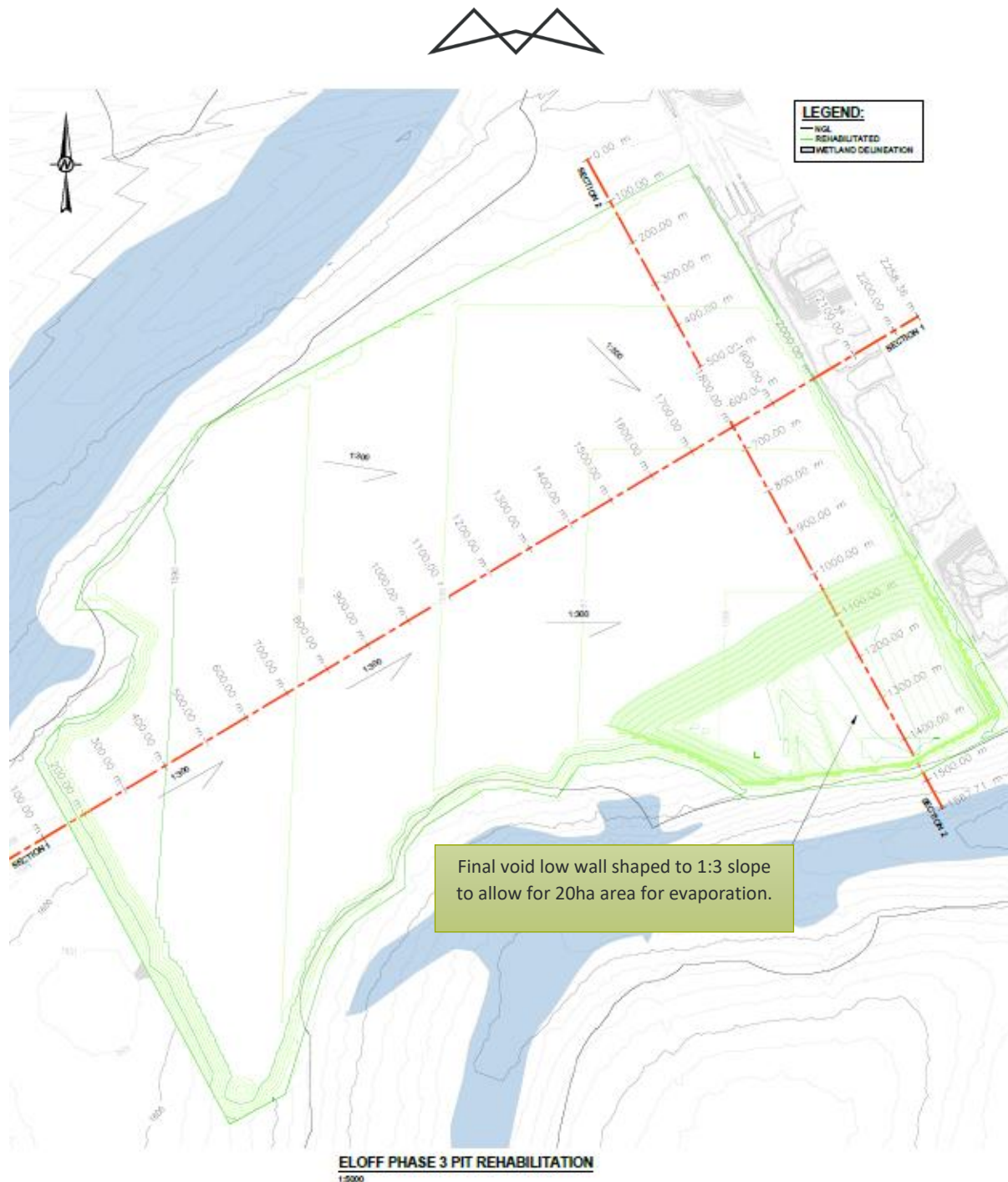
Figure 21: Option 2 – Evaporation final void/pit lake
