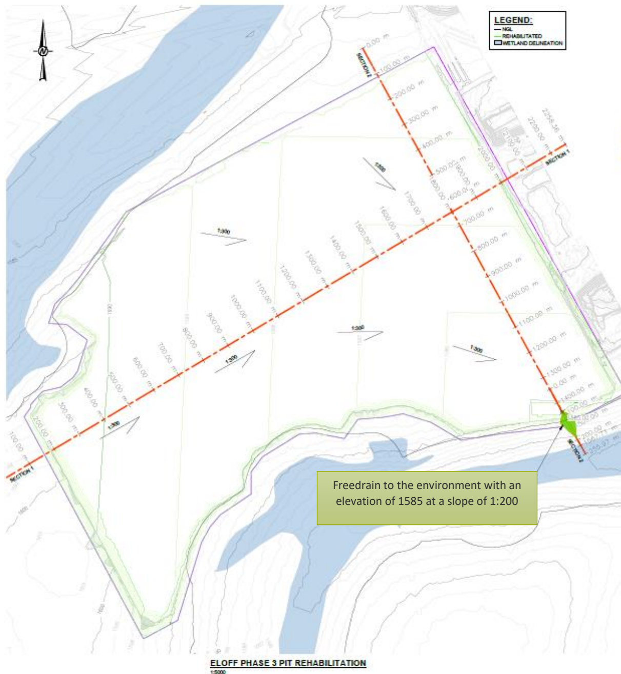
Figure 20: Option 1 – Freedrain Topography
