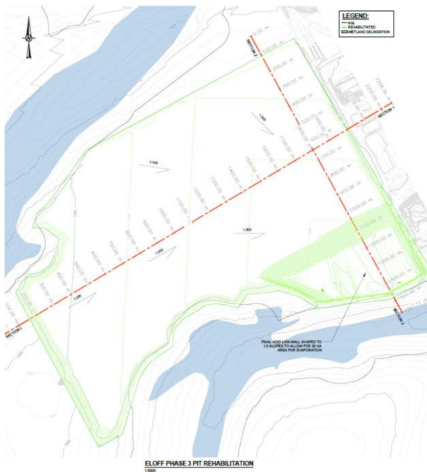
Figure 25: Option 2 – Evaporation final void/pit lake
