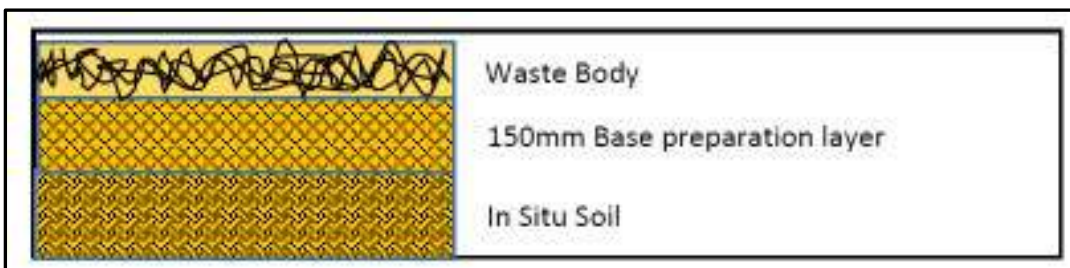
Figure 20: Proposed Class D landfill liner system
